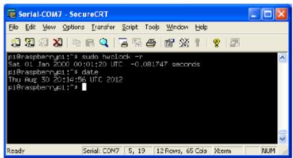
Ethernet or Wifi - it will automatically set the time from the network. Once the time is correct (check with the **date** command), run **sudo hwclo ck -w** to write the system time to the RTC
